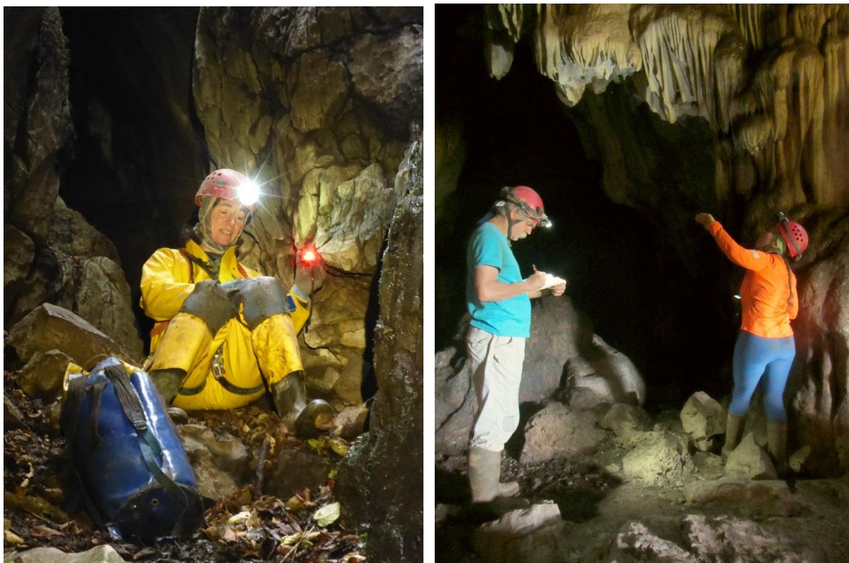
Figure 5. Cave mapping: laser range finding (left); note taking and range finding (right)
